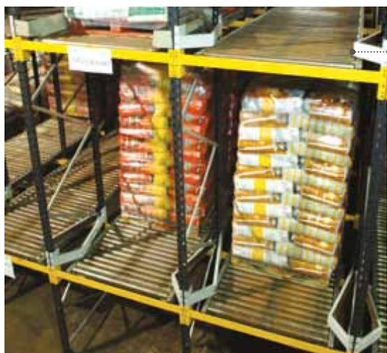
Inclined gravity rollers which are set at a fixed gradient
