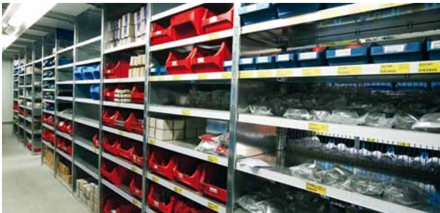
Shelf heights individually adjustable in 25 mm steps with boxes of various sizes, held in safely by mesh back cladding
