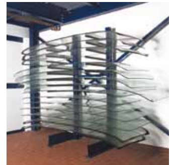
Windscreens stored on cantilever racks
