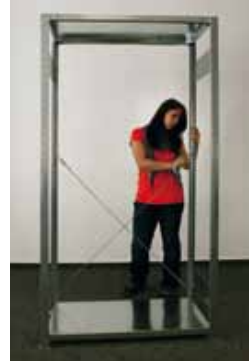
Step 4: Attach the diagonal bars and turnbuckles and straighten the shelf unit
