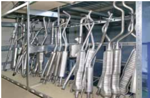
Exhaust pipes tidily arranged and separated by rod dividers
