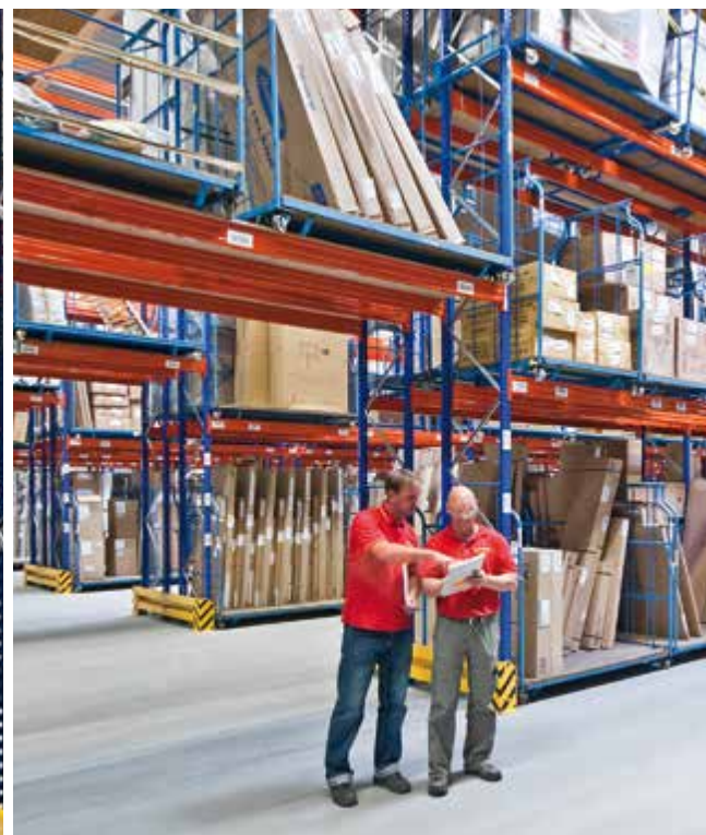
Individually adjustable rack systems make maximum use of the storage space and hold goods of various formats.
